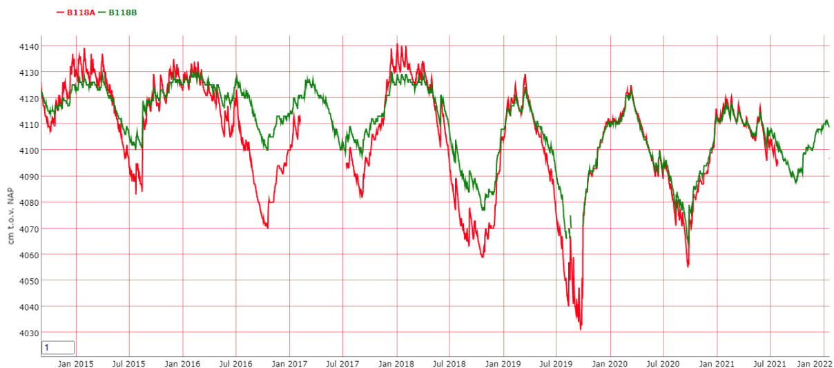
Figure 2.5.1: Example of measured groundwater level in the Witte Veen. B118B (green) is positioned in the peat layer, B118A (red) below the peat.
