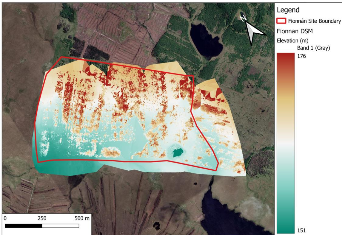
Figure 41: DEM created from drone flights at Fionnán in October 2023.
