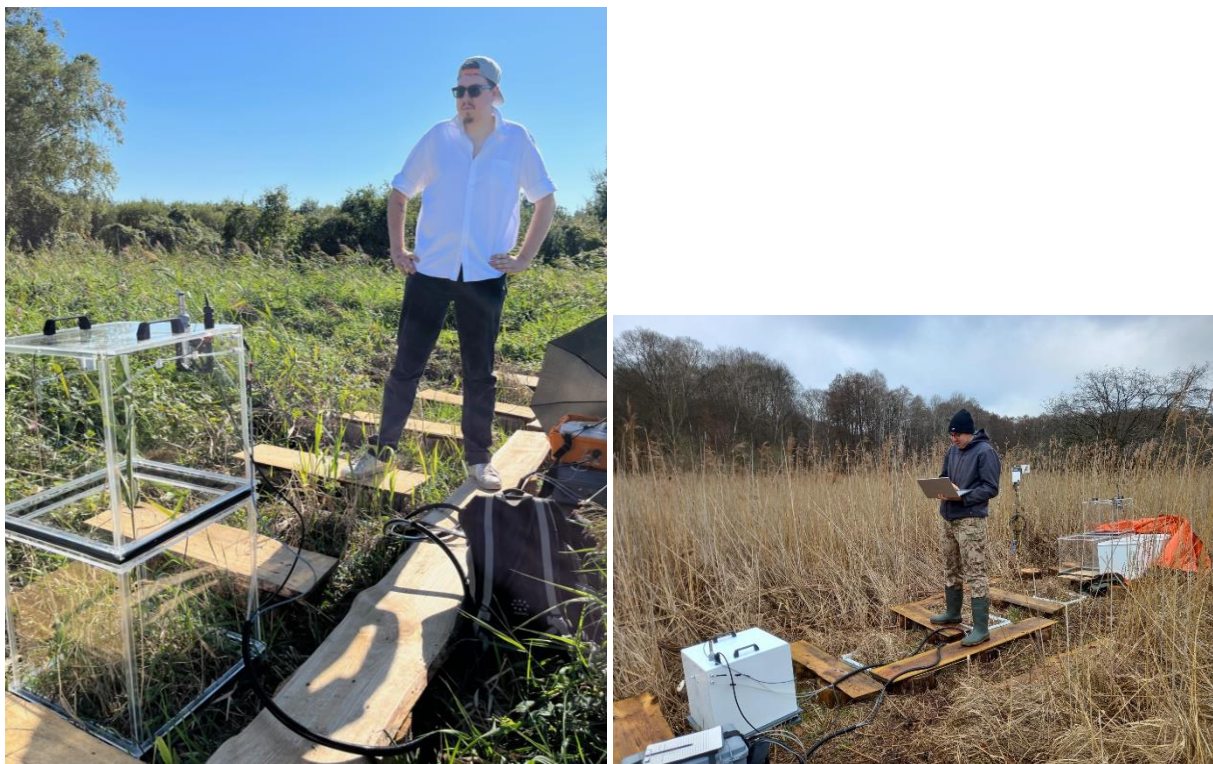
Figure 17: Boardwalk and set-up of GHG-measurements at project site "Häsener Luch" (HL01) (left), and at the reference site "Rüdritzer Fließ" (right).
