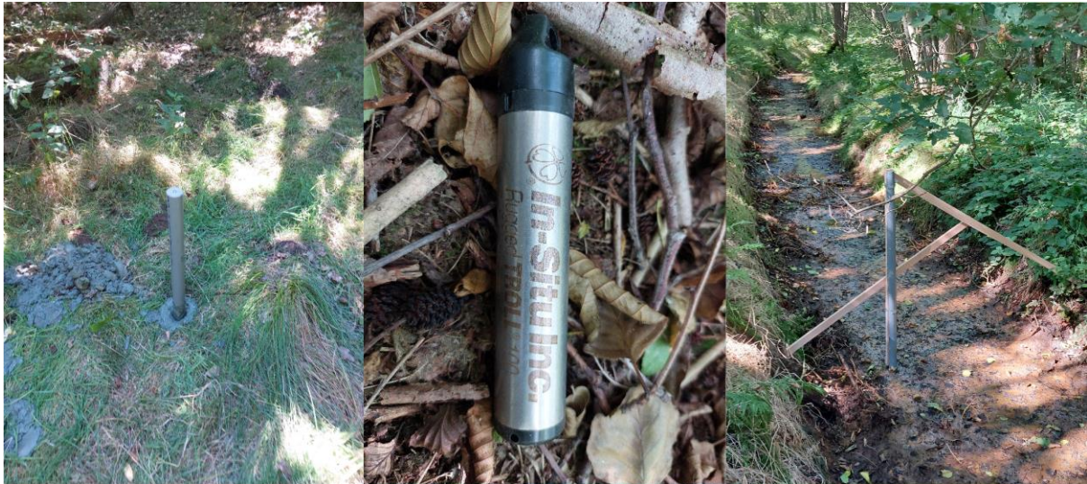
Figure 2.1.2: Installed piezometers: Left: placed in the peat soil. Middle: a datalogger. Right: placed on the bottom of the waterway
