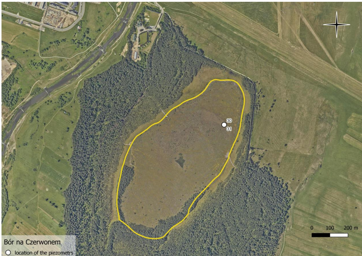
Figure 51: Location of piezometers at Bór na Czerwonem site
